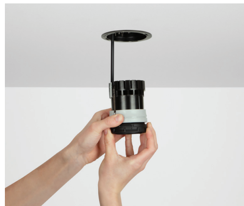
3 Lift the spring-loaded plastic lock and twist the optic and bezel from the body.
