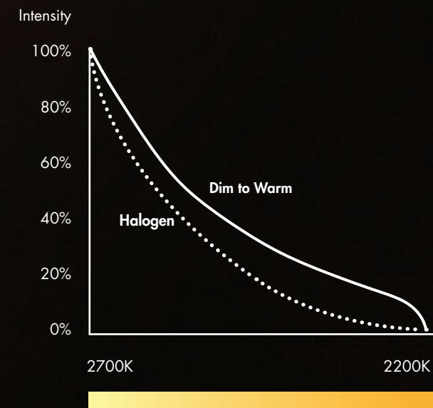
Lumenpulse Dim to Warm dimming curve compared to halogen
