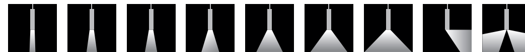
Extra narrow spot 5° Very narrow spot 10° Narrow spot 15° Narrow 25° Medium 40° Wide 60° Very wide 80° True asymmetric wallwash Double asymmetric
