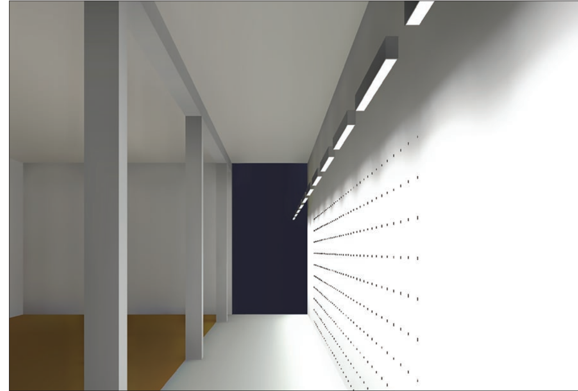
Lumenline pendant, 10 x 4 foot unit, high output (12W/ft), 3000K, Asymmetric wallwash optic, mounting height 10 ft
