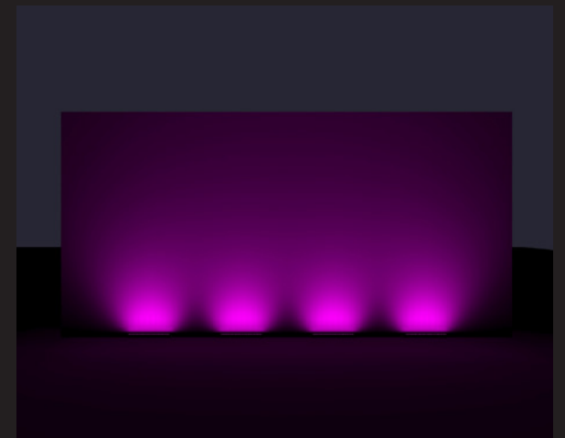
Spacing between fixtures at 1219mm.
